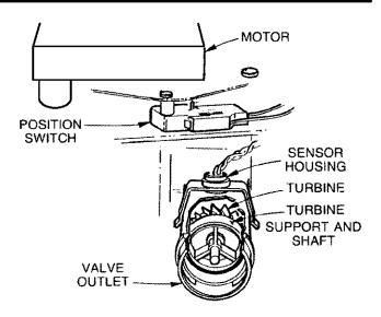
**B.** The letter (P) and dashes indicate POSITION switch operation. If the letter appears, the switch is closed. If the dashes show, the switch is open.
